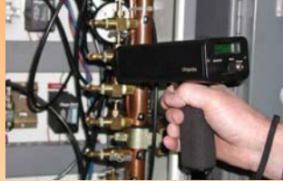
Detect air leaks
